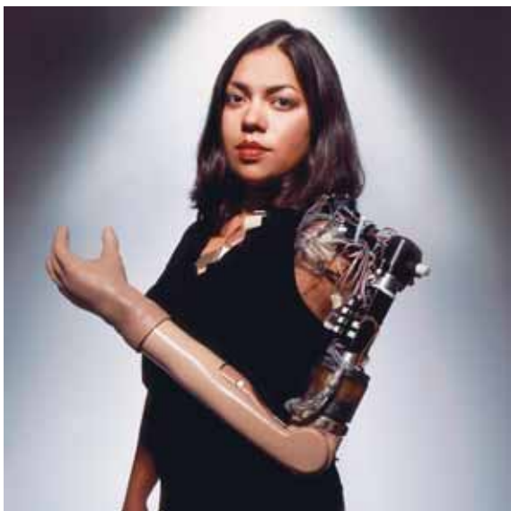
Figure 12 – Claudia Mitchell: After losing her arm in a motorcycle accident, Claudia Mitchell became the first woman to be outfitted with a bionic arm developed by the Rehabilitation Institute of Chicago. The neural prosthetic operates by detecting the movements of muscles in her chest that have been rewired to the stumps of nerves that once went to her amputated arm. Credit: Anna Knott Photography.
